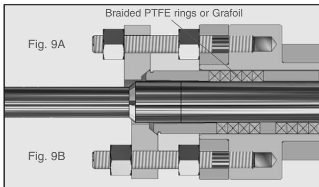
**Figure 11A: Packing: Formed Rings**
