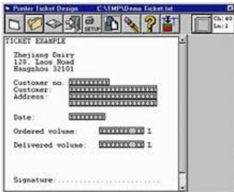
Program for design of printer tickets for the PD 4000/340 Flowmeter-Display. The program makes it possible to create a ticket layout on the PC monitor. This design is then downloaded to the PD 4000/340. A customized ticket layout may be saved on the PC hard disc for later use. Requires PD 3920/PD 3930 and VIGO software. The Printer Ticket Design Program is sold on a try-before-buy basis. Click the "files" button below to go to the download page.
