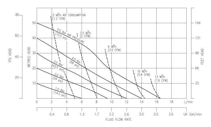
B06 Non-Metallic Pump Performance Curve, performance based on water at ambient temperature.
